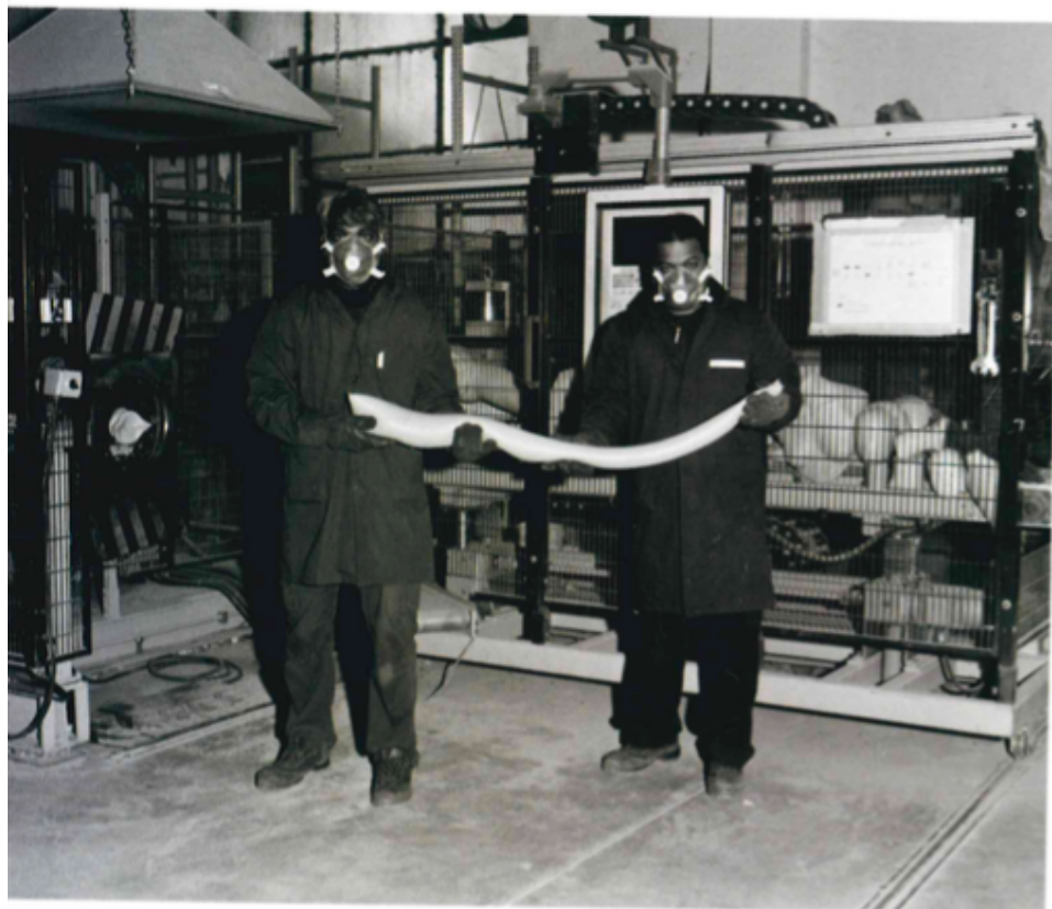
Craftsmen hold a piece of very hot plastic that has just been extruded, ready to be deposited in a mould
